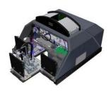
Upper and lower measurement heads are easily separated to facilitate cleaning and service of sensor windows using a convenient end column mounted key switch. The Q4000 measuring head internal temperature and relative humidity are continuously monitored, with alarms for out of range conditions. Over temperature protection circuitry will disconnect power, if necessary.
