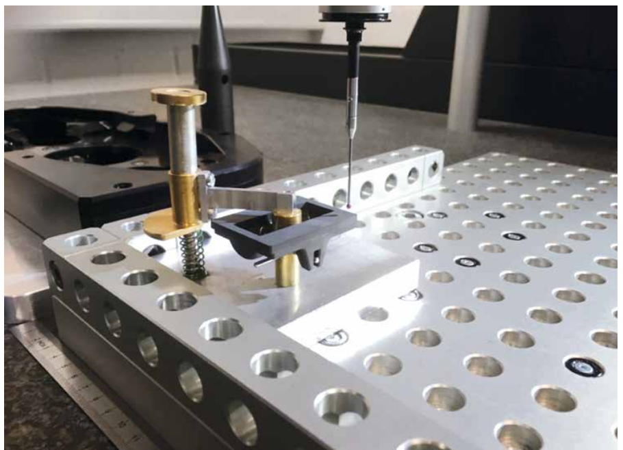
Checking of a valve slide with a 3-D coordinate measuring machine
